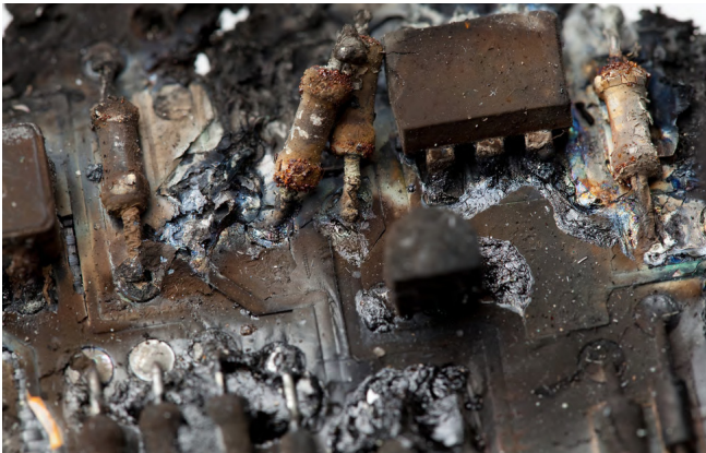
Figure 6. Circuit Board Damage Due to ESD
